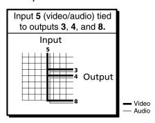
Figure 3-10 — Example 1, final configuration
